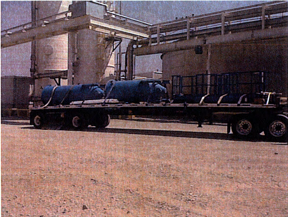
Figure 8 Parkson D2 Sand Filters (Foreground on trailer)
