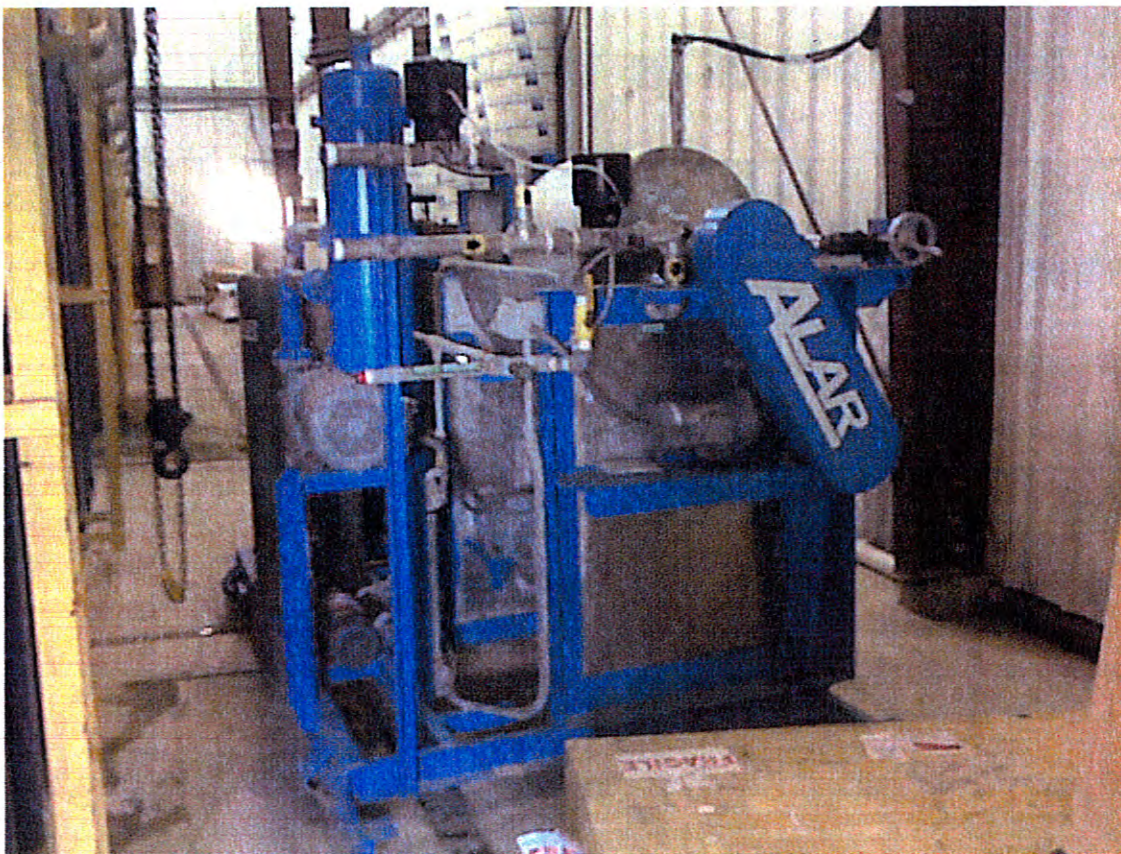
Figure 12 Alar Corp Rotary Vacuum Pilot Skid
